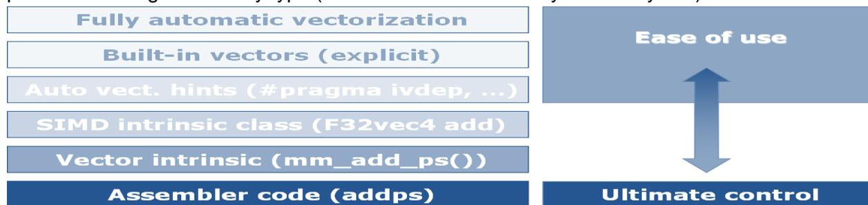
Figure 2: In contrast to auto-vectorization (e.g. applicable to `for` and `cilk_for`), an explicit way to generate vectorized code is given by built-in vectors (Cilk array notation). In contrast to user-mandated vectorization (`#pragma simd`), correct code is generated in any case rather than mandating SIMD code even against the compiler's heuristics and analysis.
